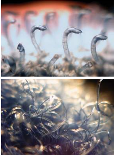
Figure D2: Magnified images of VELCRO ® showing the tiny hooks and loops
